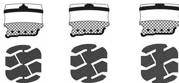
GOMMA NUOVA NEW TYRE / PNEU NEUF GOMMA SEMI CONSUMATA HALF WORN OUT TYRE / PNEU SEMI-USÉ GOMMA CONSUMATA WORN OUT TYRE / PNEU USÉ
